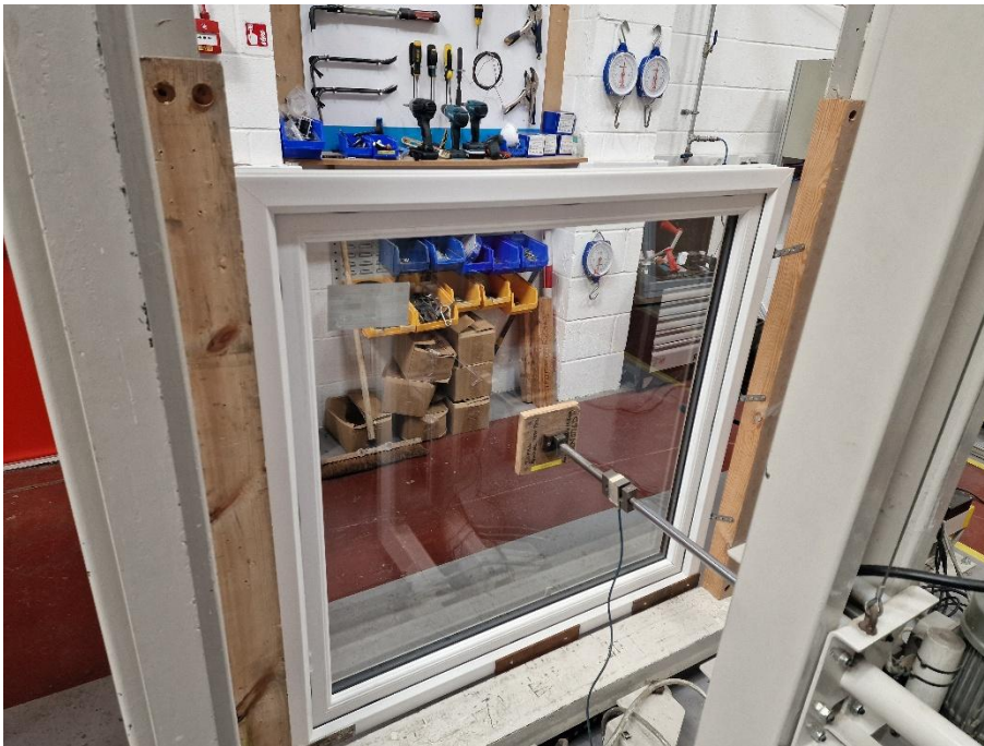
Figure 1: Central load preload being applied.
